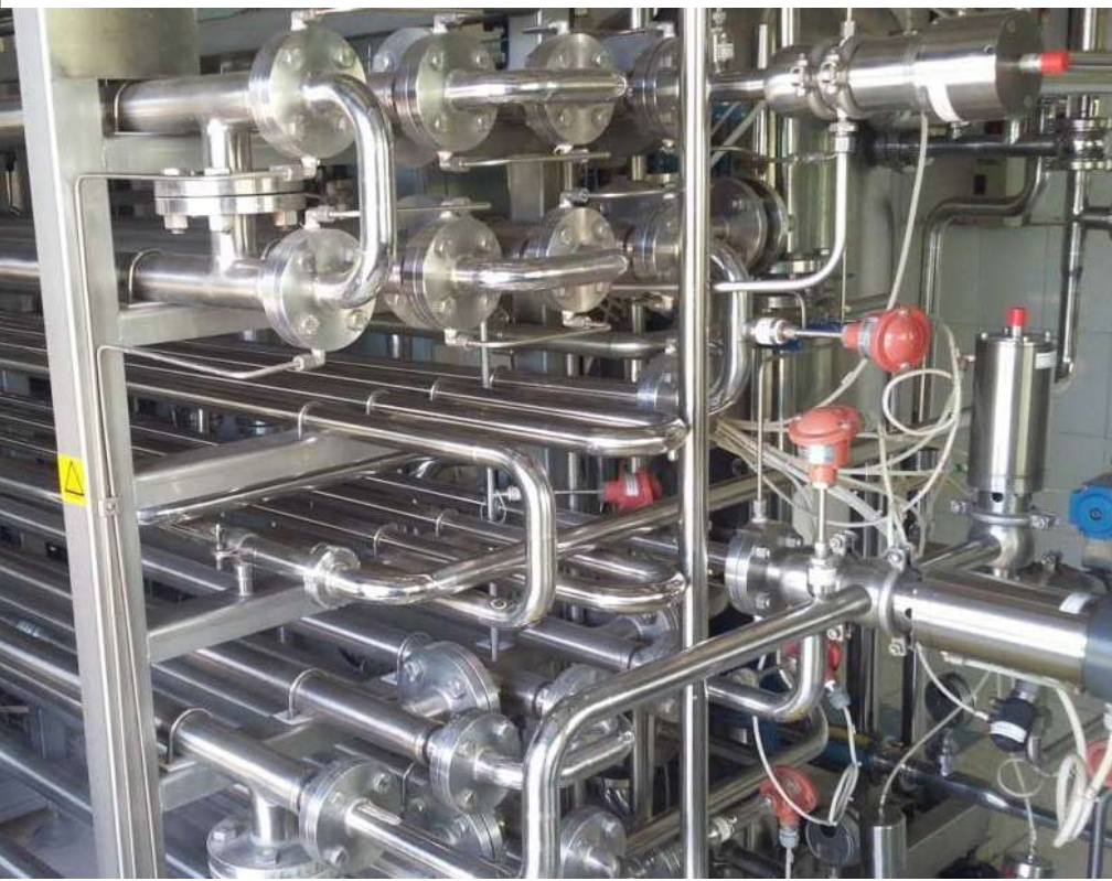
ABOVE: Mango pulp sterilizer. BELOW: Mangoes at the ripening facility at MNJP in Malindi.
